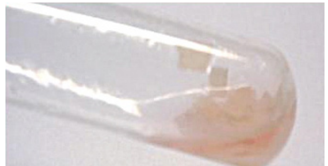
Membrane oxidation damage
